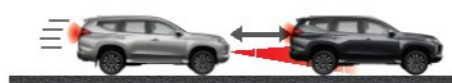
When the vehicle in front slows or stops, ACC slows or stops your vehicle.
