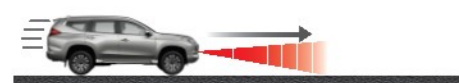
Your selected speed is maintained even if you remove your foot from the accelerator pedal.
